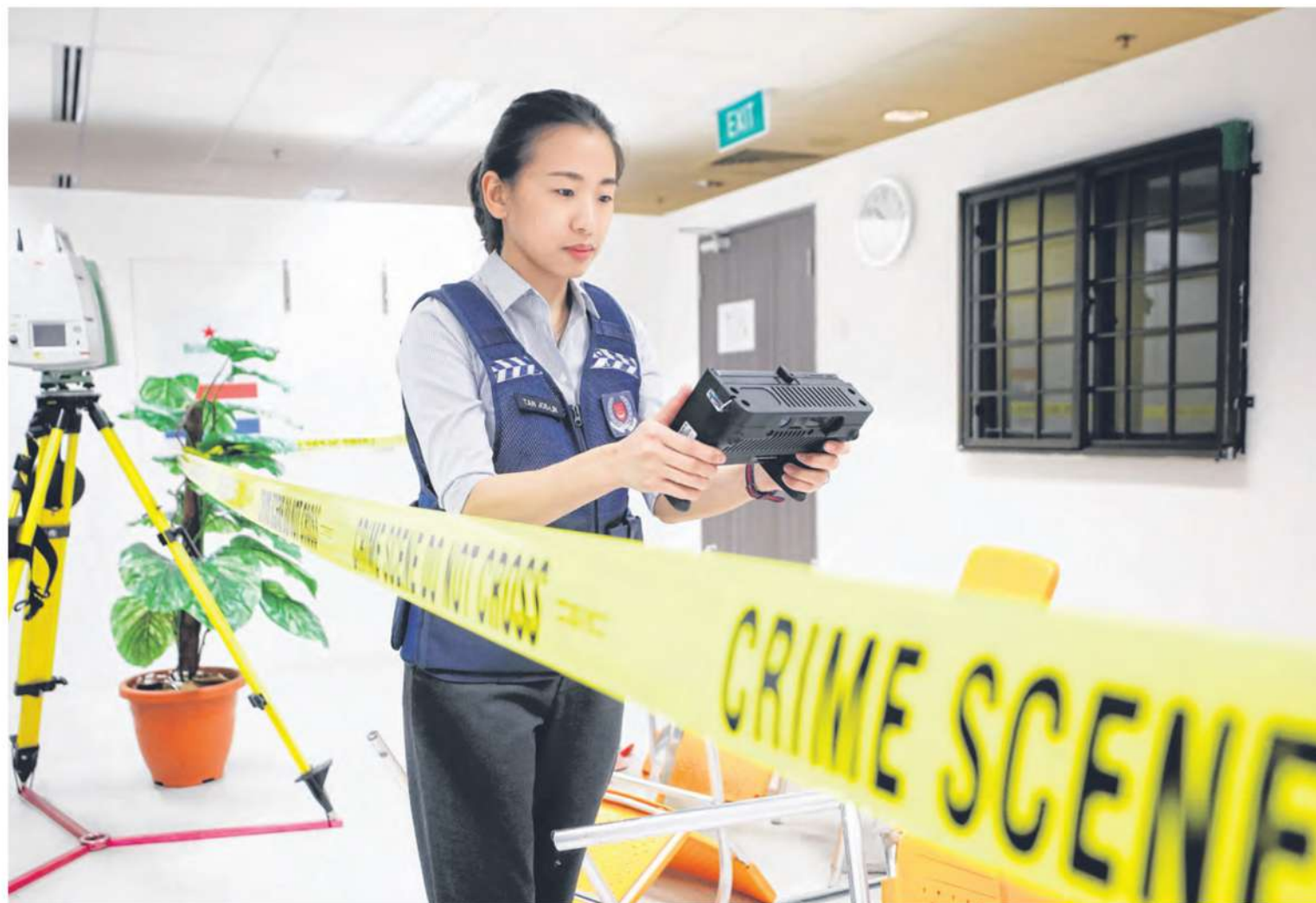
Ms Tan Joe-Lin, who supervises a team of crime scene specialists, using a handheld 3D scanner that is used to document crime scenes. The scanner can examine hard-to-reach places and the user can immediately see what was scanned and redo it if need be, reducing the time taken to process a scene. ST PHOTO: GAVIN FOO
